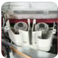
Pre-milling unit perfect joint line
